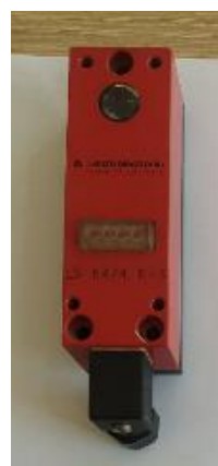
4-rasm. Nur tarqatgich optik sensor LS 64/2.8.
